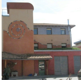
The south side of Pamplona's house has large openings but is protected by sun shades so that heat and light can be controlled depending on the season.
